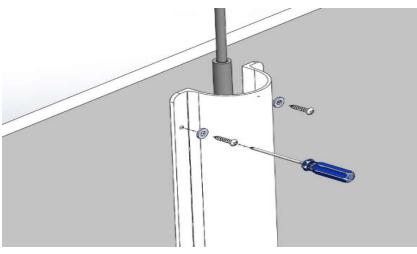
**Step 2:** Fasten the Cord Protector to the divider using supplied screws / washers.
