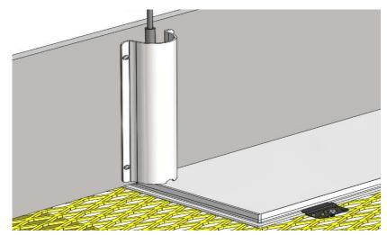
Image of cord protector properly installed
