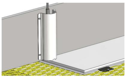
Image of cord protector properly installed
