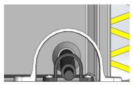
**Step 1:** Position cord protector over cable / conduit. Be sure to leave equal space on both sides of connector.
